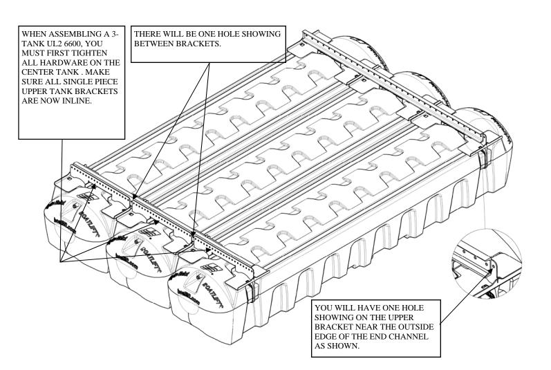
> End Channel Keel Spanner Assembly Fig. F
